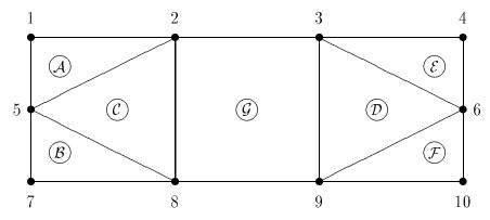
A matrix can be associated with each element. Each has nonzeros only in the rows or columns associated with variables at the nodes of the given element. If we choose numerical entries for the nonzero entries in the element matrices to be 1.0 on the diagonal and -1.0 for the off-diagonals, then the element matrix corresponding to the element labeled  ${\cal A}$  is the  $10\times 10$  matrix:
